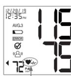
Movement, shaking, or talking during the measurement can result in pulse irregularities that may cause the appearance of this icon. Therefore, it is of great importance to not move or talk during measurement.
