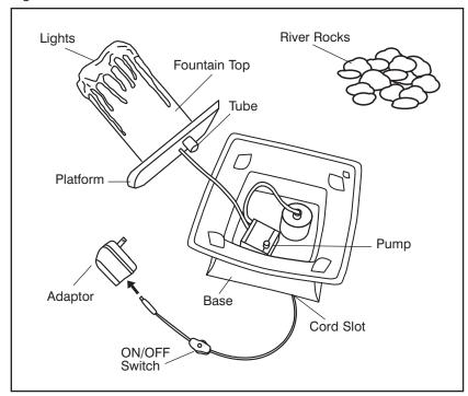
3. Insert the pump into the tube on the bottom side of the fountain top (Fig. 2).
