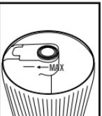
3. Fill with clean, cool water or distilled water (if in area with hard water) until the water level reaches the MAX fill line. DO NOT fill with warm or hot water. **CAUTION:** Never add essential oils or other additives to the water tank or water reservoir. Refer to the section on how to properly use essential oils with this humidifier.
