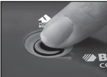
Occasionally, if sheet capacity is exceeded or if the paper is not put in straight, you may experience a jam. Black & Decker developed **Power Boost Technology that provides an overdrive function to power through a paper jam.**
